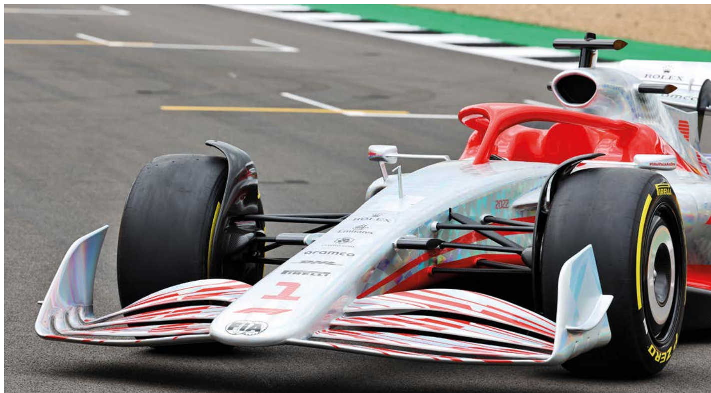
The increase in tyre diameter from 660mm to 720mm has broad design implications, as does the greater distance between the brakes and the new wheel rims
