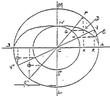
follows: Draw two circles around one common centre C. The radius of the first (CA) represents one half the size of the major axis AB of the ellipse to be constructed and the radius of the second circle CN represents one half of the ellipse we intend to construct. Both of these axes are known.
